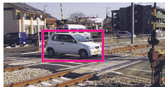
Camera Image of Road (Detected results are displayed in red frames in camera images)
